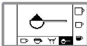
During preparation of coffee with pre-ground coffee, the "ground coffee quantity" function is deactivated. Therefore no information on the ground coffee quantity appears on the display.
