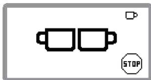
You can switch between one cup or two cups during the grinding process by pressing the **OK** button.
